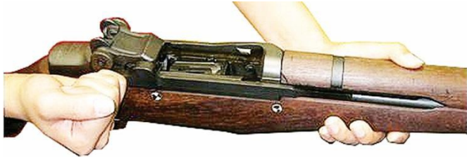
Figure 1. Pulling operating rod
