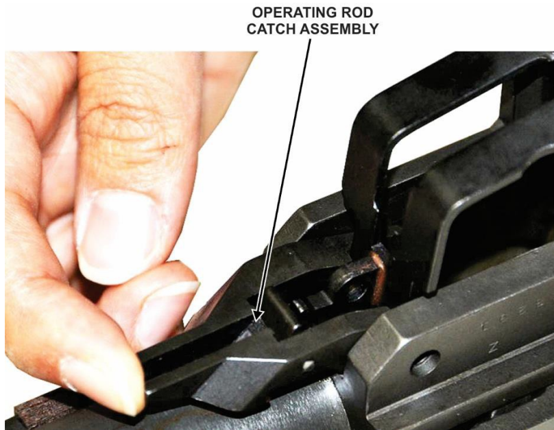
Figure 46. Testing operating rod catch assembly
